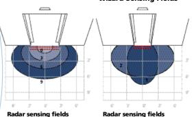
Radar sensing fields in accordance with sensitivity settings (tilt angle 27° with wide antenna) Safety curtain (tilt angle 0° with wide lens cover)
