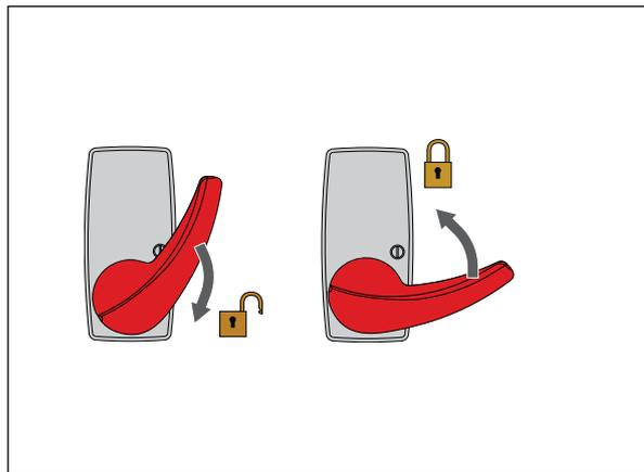
In the event of maintenance, malfunctioning or emergency, pull the lock release lever VALSB down and turn it to the right or lower the lock release lever LOKSBM (if installed) and move the door wings manually into the open position.
