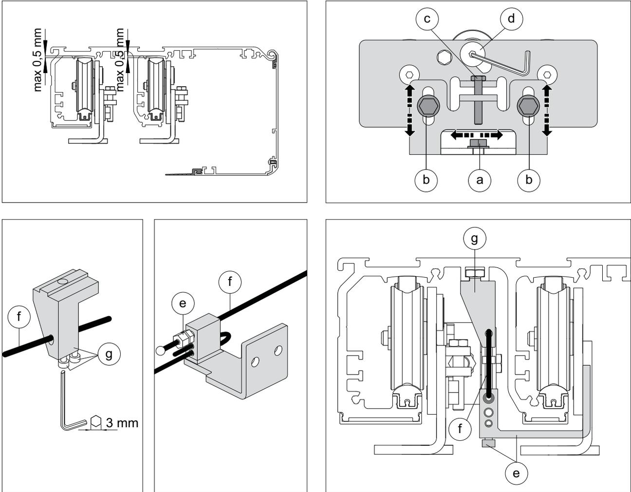
Make sure that the central wheel is adjusted [d] as illustrated in the diagram.
