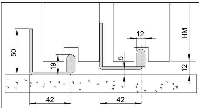
The floor guide for the PAMH60 door wing has the measurements indicated in paragraph 5.3.
