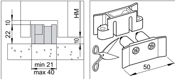
The measurements of the code KPAM45 floor guide for telescopic door wings are indicated in the diagram.
