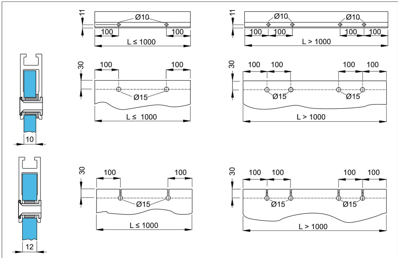
The diagram indicates the process measurements of the aluminium profile AC4255 and glass.  $\text{Ø}6,5$  countersink  $3 \times 45^\circ$  through holes are required on the aluminium profile and  $\text{Ø}15$  on the glass for fastening. The number of holes and related distance between centres are based on the door wing width.
