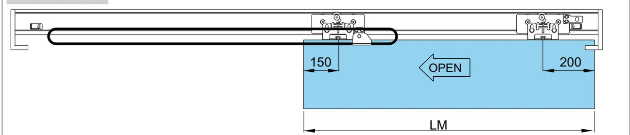
Make sure that the central wheel is adjusted [d] as illustrated in the diagram.
