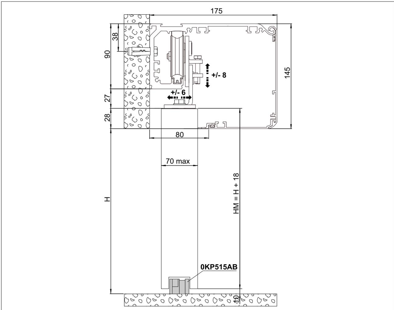
Unless otherwise specified, all measurements are expressed in millimetres (mm).
