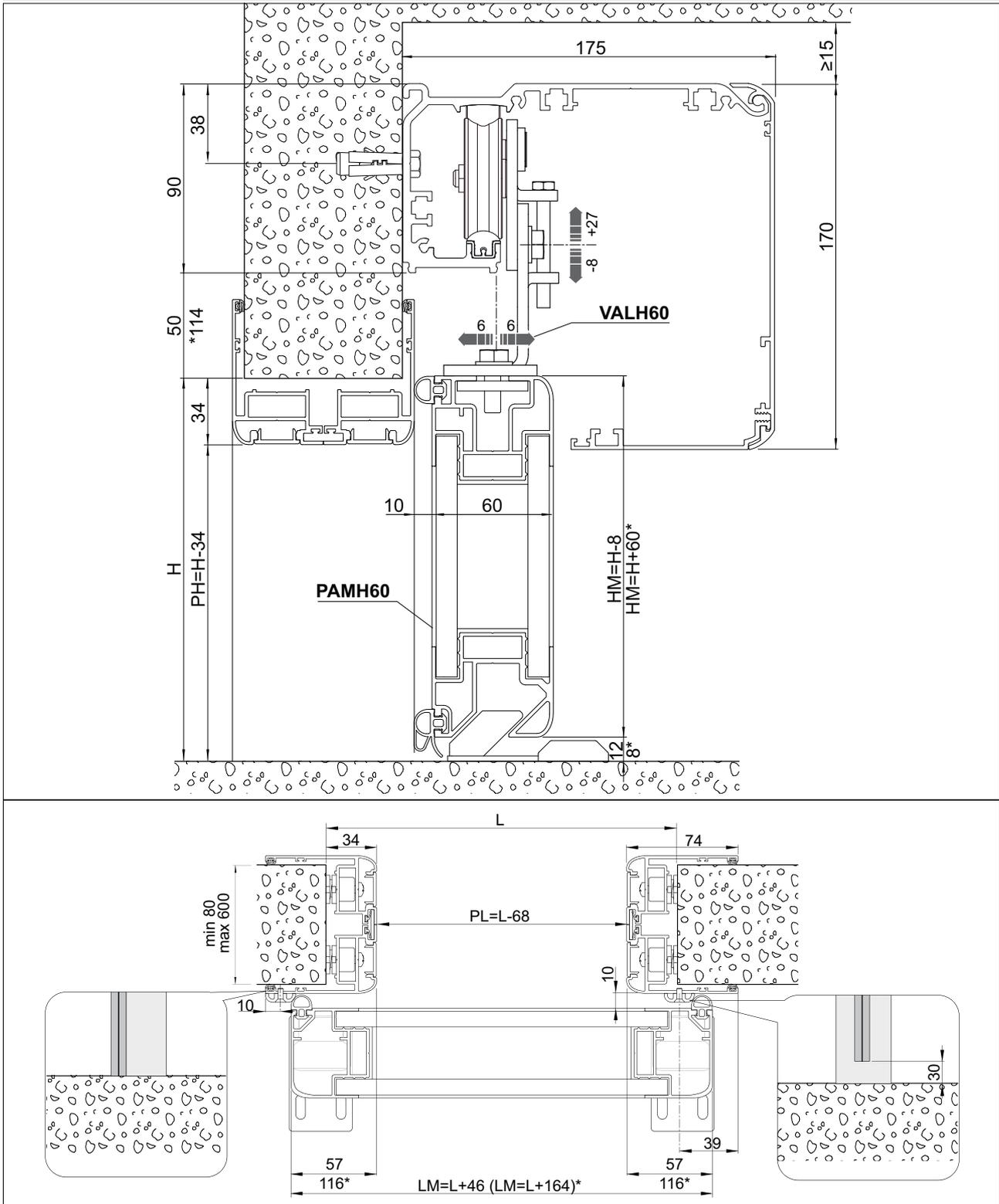
Unless otherwise specified, all measurements are expressed in millimetres (mm).
