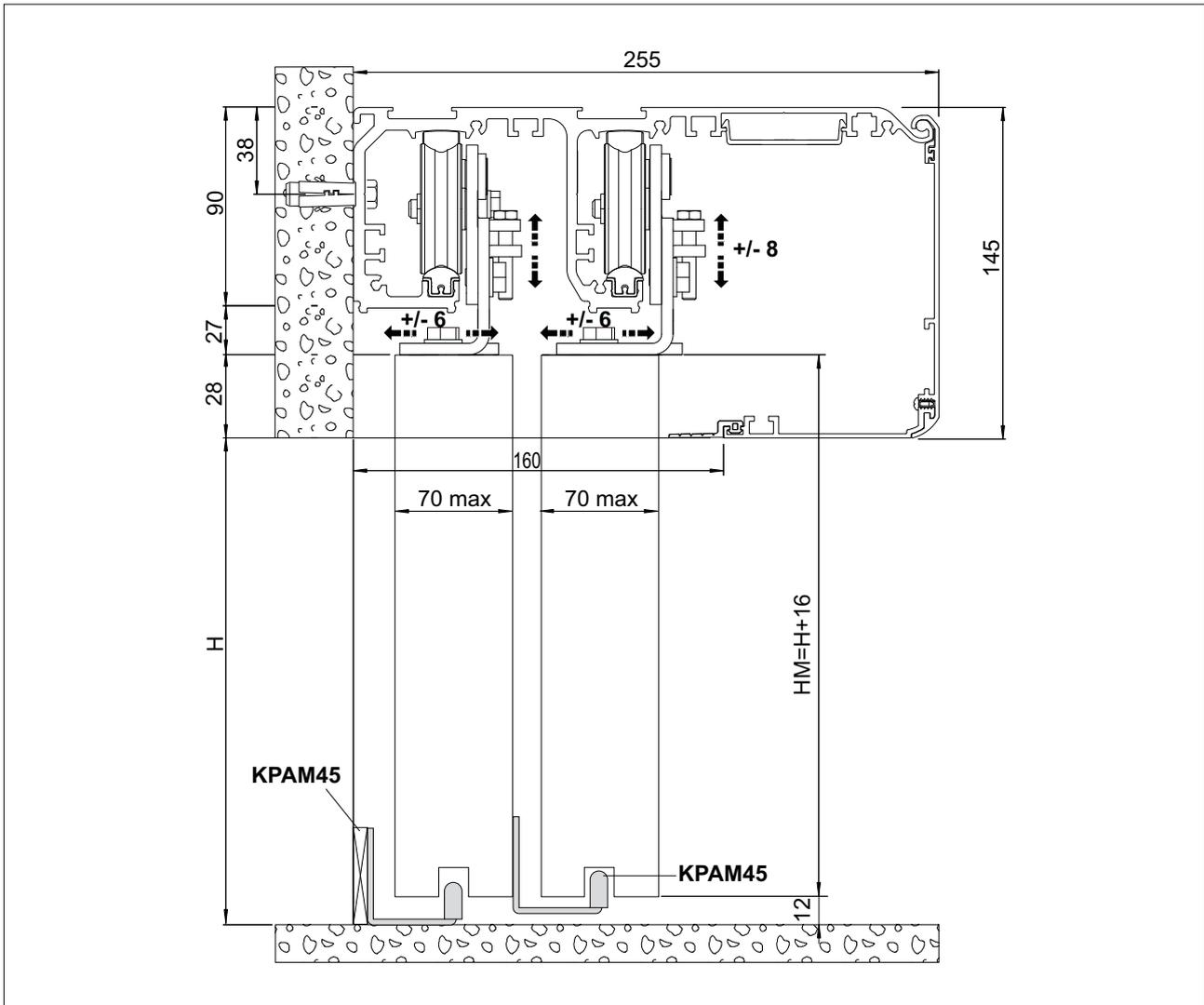
The VALOR T automation wall fixing measurements are illustrated in the diagram, considering that the door wing profiles are not of our production.
