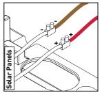
Connect the 24V solar panel cables = (not supplied), the negative to the brown wire (-) and the positive to the red wire (+).
